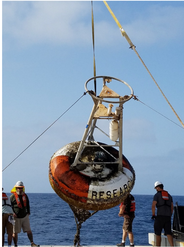
FIG. 4 Recovery of a moored PIRATA buoy during an NOAA PNE/AEROSE (Section 5.1) campaign. Shown in the photo are the buoy's surface float and tower. The meteorological sensors, which were attached to the tower when deployed, have been removed. A thick rope attached to the tower through a pulley on the A-frame keeps the surface float suspended until the line of oceanographic sensors below the float can be secured to the deck. Smaller lines attached to the tower and A-frame keep the buoy secure. Note that the surface float is covered with dust aerosols (from the Sahara) on the top and marine life on the bottom.
