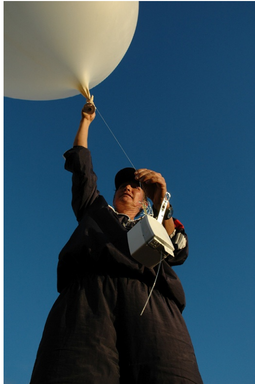
FIG. 1 Meteorologist launching a radiosonde at San Cristobal, Galapagos, Ecuador.
