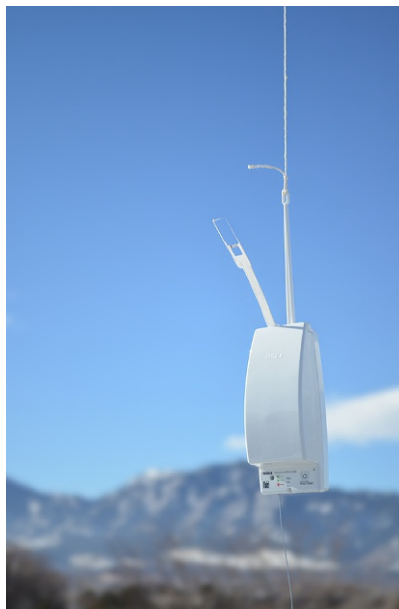
FIG. 2 Radiosonde with temperature and humidity sensor boom extending up and out.
