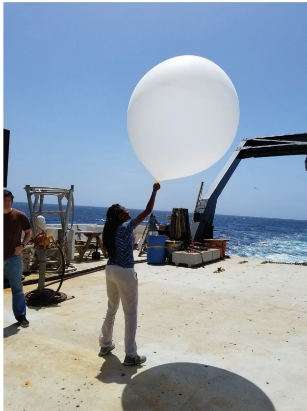
FIG. 3 Launch of a satellite-dedicated radiosonde from the fantail of the NOAA Ship Ronald H. Brown while underway, timed approximately 15–30 min prior to a forthcoming 13:30 SNPP LEO satellite overpass. Pictured is Howard University student Kafayat Olayinka with the radiosonde package (left hand) and a 200 g helium-filled balloon during a joint NOAA PIRATA Northeast Extension (PNE), Aerosols and Ocean Science Expedition (AEROSE) campaign (Section 5.1).
