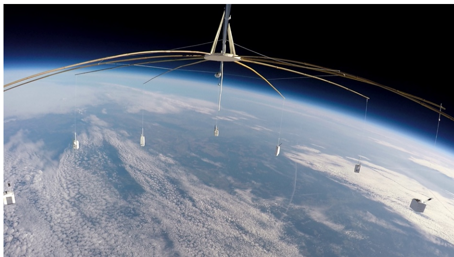
FIG. 10 Screenshot of a camera recording of a test flight with a rig carrying 10 radiosondes, that will be employed for the 2022 radiosonde intercomparison campaign.
