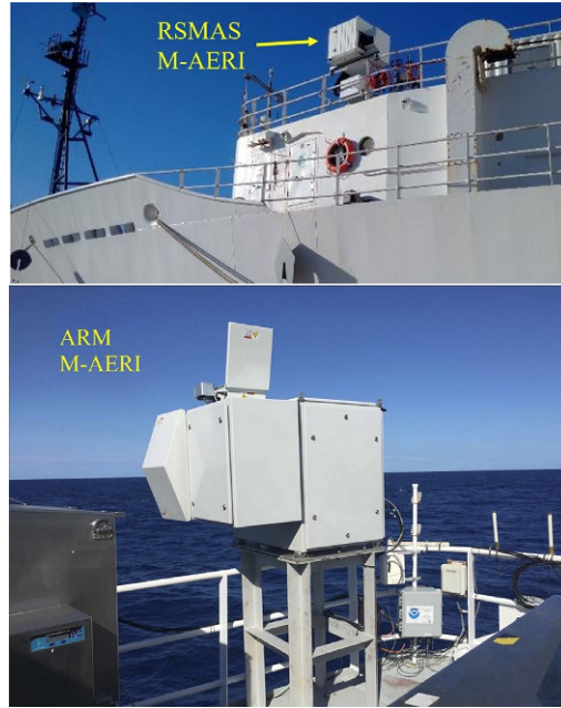
FIG. 5 The third generation RSMAS M-AERI (above) and the ARM M-AERI (below) installed on the NOAA S Ronald H Brown . Lower image courtesy of the U.S. Department of Energy of Atmospheric Radiation Measurement (ARM) user facility.
