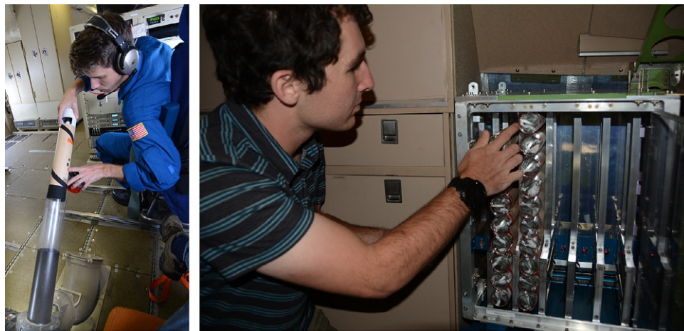
FIG. 2 (Left) Manual dropsonde launch onboard the NOAA WP-3D research aircraft. (Right) Automated dropsonde launcher onboard the NSF/NCAR GV research aircraft.
