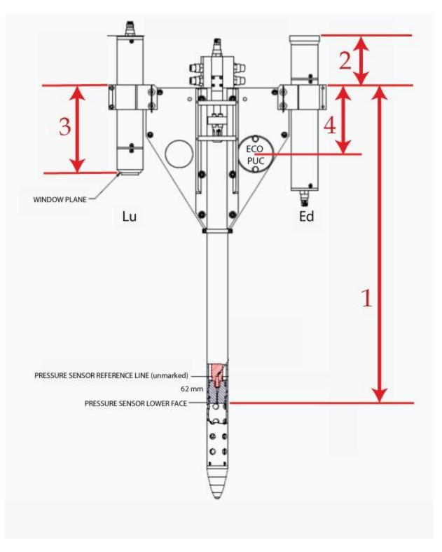
Measurements required to derive the sensor distance offsets. This is an edited version of a figure from the Operation Manual for the Profile II, revision K, 10 December 2012.
