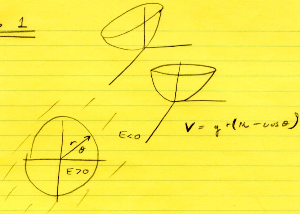
$$E = \underbrace{\frac{1}{2}(1+\mu)\dot{r}^2 + r^2\dot{\theta}^2}_{\text{post definite}} + gr(\mu - \cos\theta)$$
